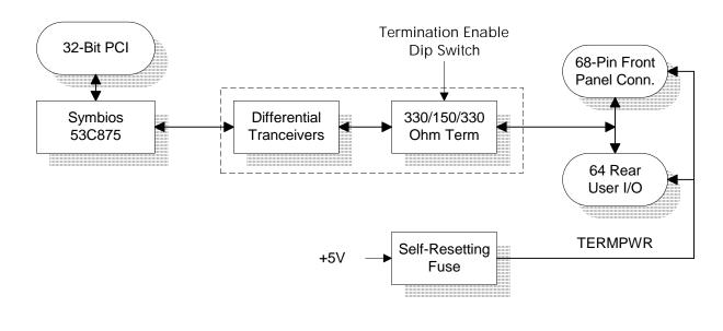
The SCSI PMC adapter from Technobox interfaces a host board PCI bus to a standard SCSI interface via a 53C875 controller.
