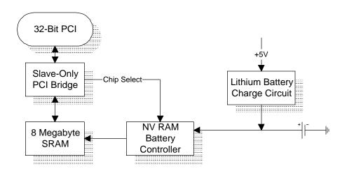
The Non-Volatile SRAM PMC provides a means for reliably storing up to 8 Megabytes of random access data for at least 2 months during power down.
