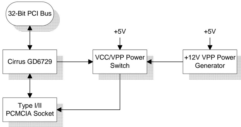
The Technobox PCMCIA to PMC Adapter permits use of PCMCIA cards in a PMC slot.
