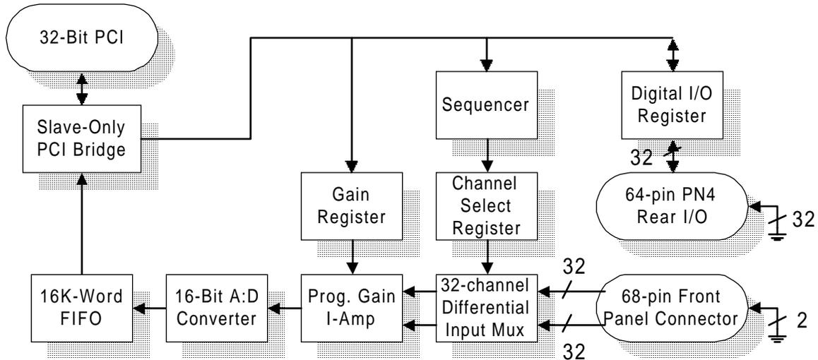
The 32-channel, 16-bit A:D converter card from Technobox provides a combination of digital and analog interfaces on a single-wide PMC.
