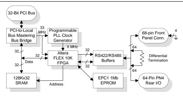
The 32-channel Reconfigurable RS422/RS485 Digital I/O PMC provides a vehicle for implementing complex user-specific digital designs requiring a differential interface.
