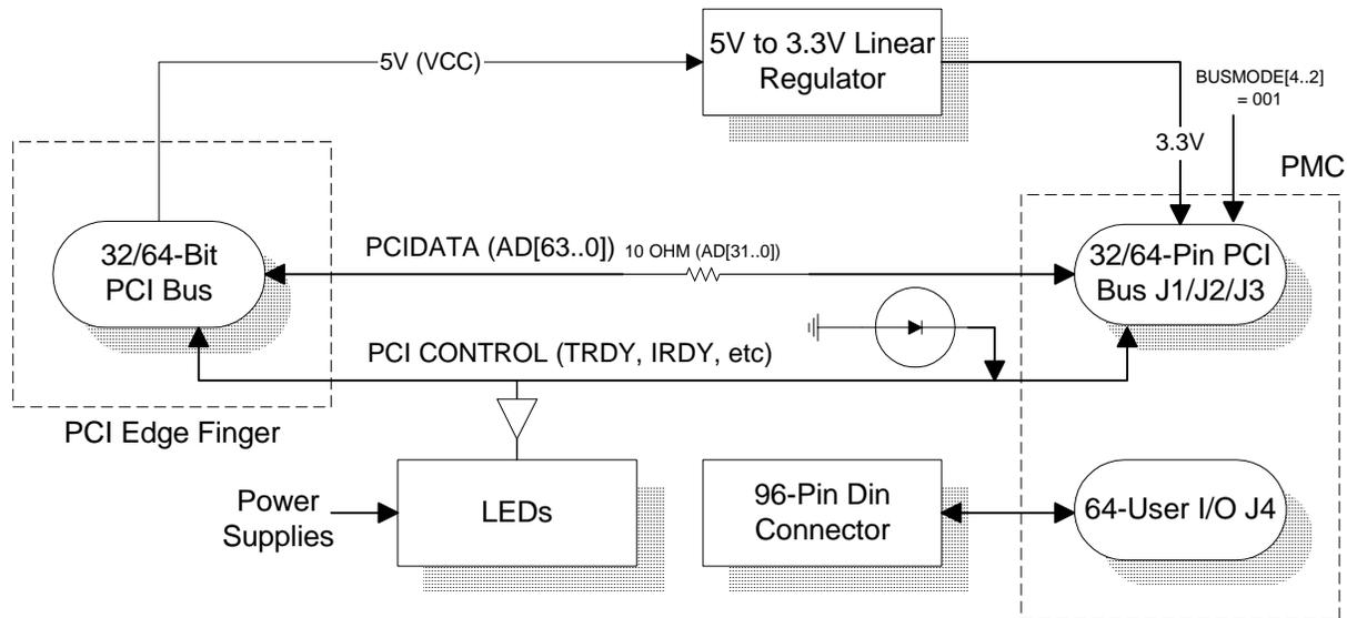
This 64-bit PMC to PCI Adapter permits delivery of PMC-derived applications in a standard PCI environment.
