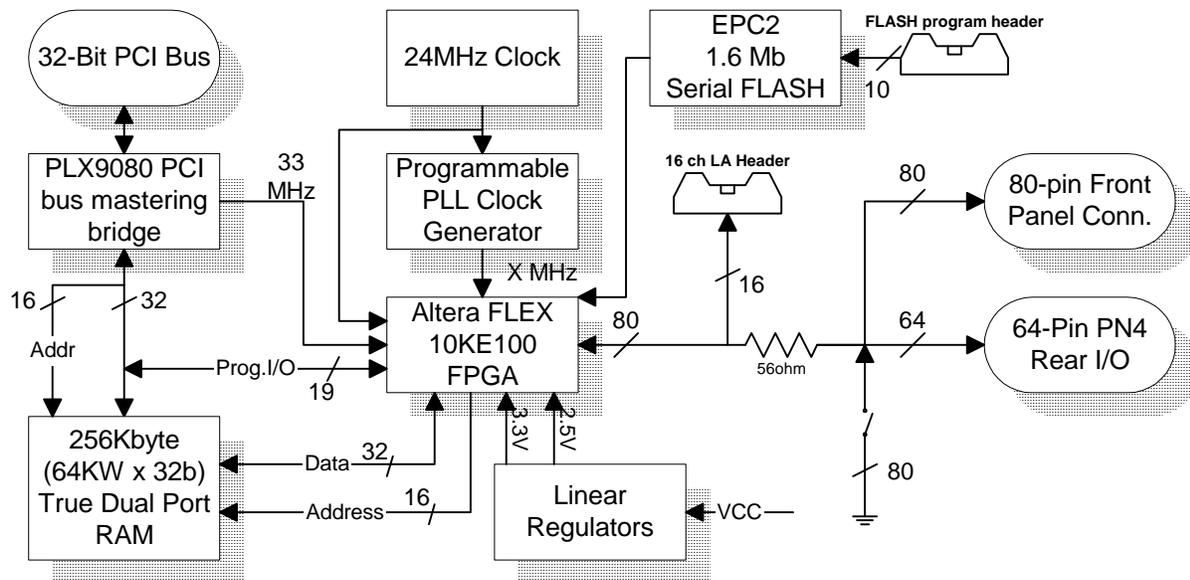
The 80-channel Reconfigurable Digital I/O PMC provides a vehicle for implementing complex user-specific digital designs requiring high speed single-ended operation. 64 of the 80 signals are available out the PN4 connector, while all 80 signals are wired to the front panel connector.
