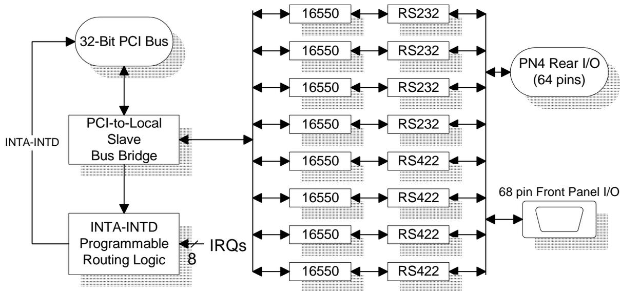
The Technobox 8-Port Async Communication adapter provides eight 16550-based UARTS, with four ports using RS232 signal levels, and four ports using RS422 signal levels.
