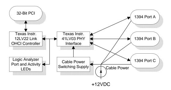
The IEEE P1394 PMC from Technobox provides 100 Mb/s, 200 Mb/s and 400 Mb/s 1394 serial bus interface with connectivity for up to three 1394 ports.
