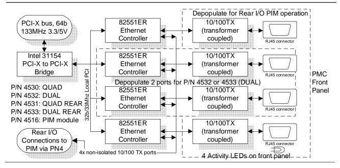
The Dual/Quad 10/100-TX Mb/s Ethernet PMC-X (per VITA 39) Adapter provides up to four Ethernet connections over twisted pair media. Options are available for Front-Panel RJ45 accessibility, or Rear I/O accessibility via a VITA 36 PIM module.
