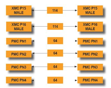
Signals are passed one-to-one between the host/carrier board and the paired PMC or XMC. This illustration represents a socket saver with all PMC and XMC connectors installed, such as Technobox P/N 7648. Assorted socket saver configurations can be created based on population options.
